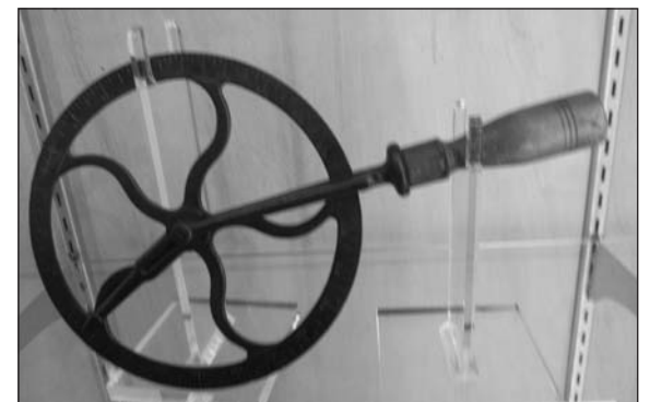
No, this was not used to cut slices into an extra large pizza. This wood and iron object, called a “traveler” was used to measure the circumference of wooden wagon wheels.
